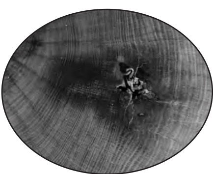
Detail of the cross-section showing links from a chain fence embedded around 1945.
